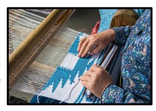
Weaving is one of the primary methods of textile production and it involves interlinking a set of vertical threads with a set of horizontal threads. The set of vertical threads are known as warp and the set of horizontal threads are known as weft.
